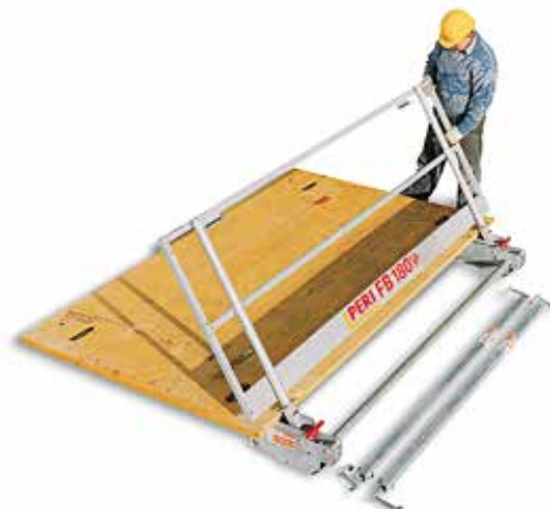
Due to its 2.40 m width, the intermediate platform can be loaded crosswise thus saving on space. The stacking height of an individual intermediate platform is only 9 cm; for nine elements, this results in a stacking height of 81 cm.
