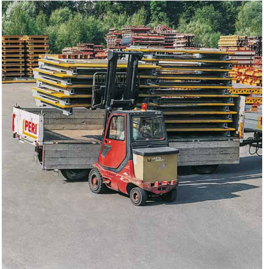
Due to its 2.40 m width, the intermediate platform can be loaded crosswise thus saving on space. The stacking height of an individual intermediate platform is only 9 cm; for nine elements, this results in a stacking height of 81 cm.
